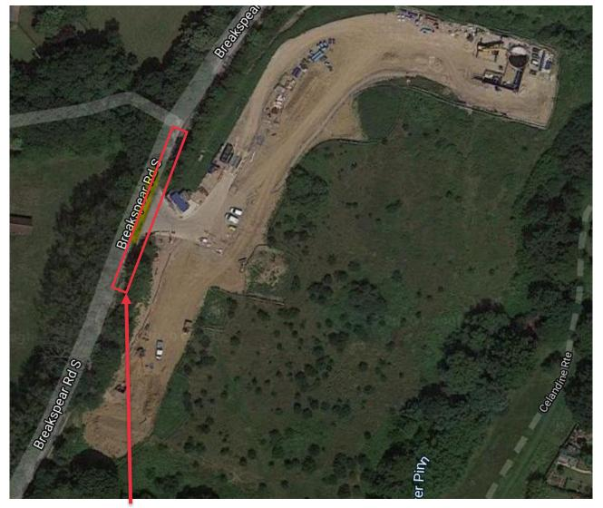
Area of work and traffic management. The south bound lane will be closed with temporary traffic lights in place at either end for the duration of the work over three days.
